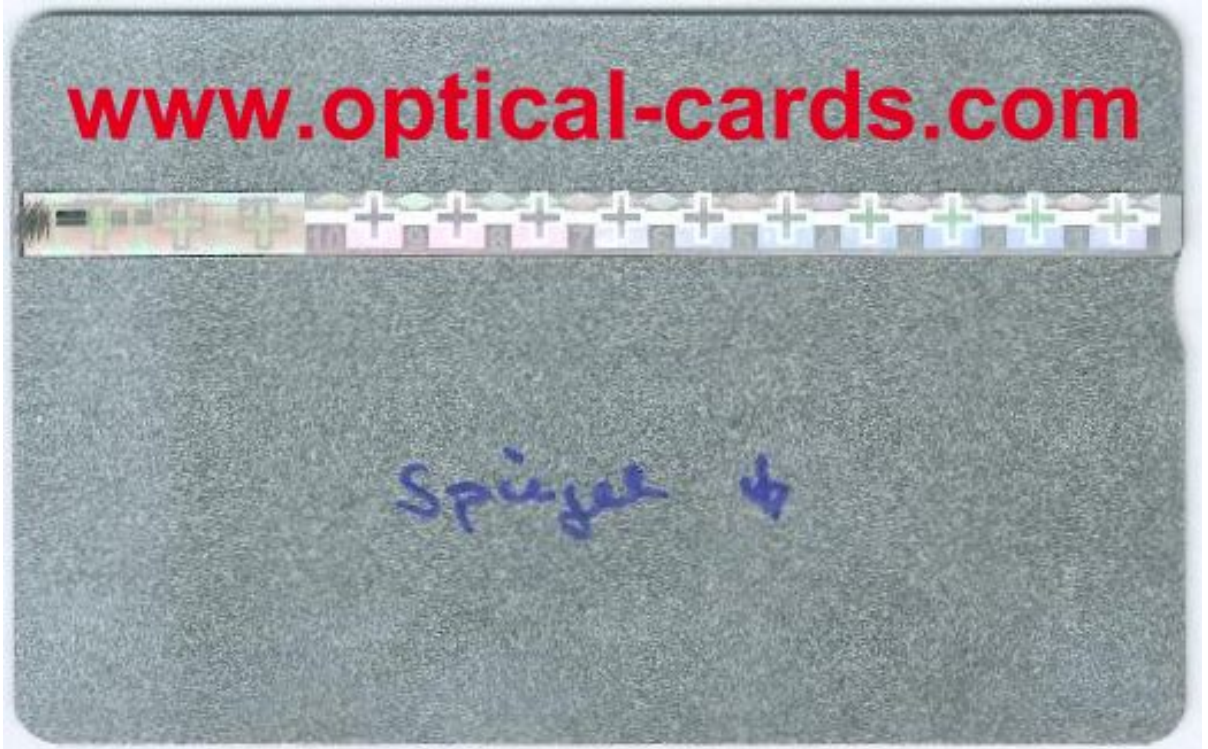
Experimental-card with opto-kinegram in order to hide the optical structure
